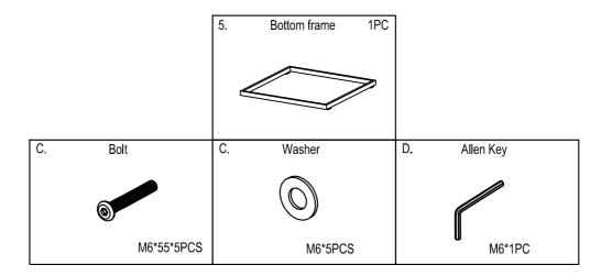
Attach bottom frame (5) to left arm (2) and right arm (1) using bolt (C) with washer (D).
